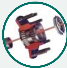
TB series trailer axles with unitized hubs
